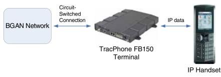
When connected to the terminal the IP handset provides a dedicated BGAN menu with a subset of the terminal configuration options.
